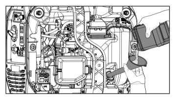
5. Check engine oil level before each use and add as needed.
