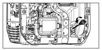
4. Tilt the generator on its side and allow the oil to drain completely.
