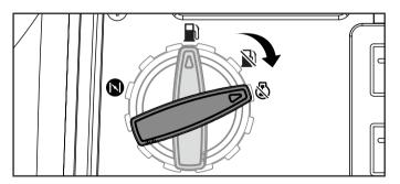
**Important:** Always ensure that the EZ Start dial and fuel vent lever are in the "OFF" position when the generator is not in use.
